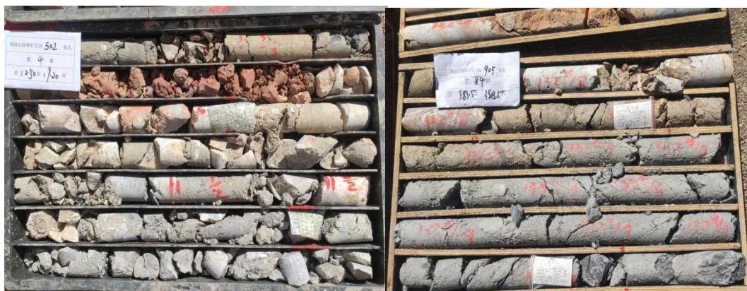
1.3-6 ZK502 钻孔中断层破碎带
